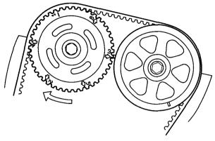
11. Rotate the crankshaft 120° clockwise (camshaft pulley turns 60°). Check that the front intake camshaft pulley is positioned as shown.
