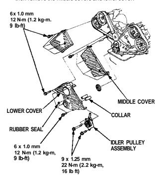
18. Loosen the adjusting boll 180° turn. Push the tensioner to remove tension from the timing belt, then retighten the adjusting bolt.
