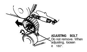
19. Remove the timing belt from the pulleys.
