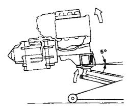
**14.** Remove the alternator bracket stiffener and dipstic pipe.
