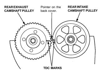
4. Install the timing belt tightly in the sequence shown.
