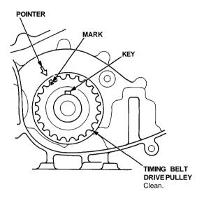
Set the front camshaft pulleys so that the No. 1 piston is at TDC. Align the TDC marks on the front exhaust camshaft pulley and front intake camshaft pulley to the pointer on the back cover.
