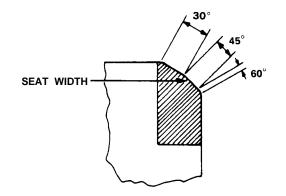
5. After resurfacing the seat, inspect for even valve seating: Apply Prussian Blue compound to the valve face, and insert valve in original location in the head, then lift it and snap it closed against the seat several times.
