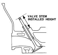
8. If valve stem installed height is over the service limit, replace the valve and recheck. If still over the service limit, replace the cylinder head; the valve seat in the head is too deep.
