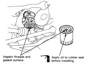
4. Start the engine, and check the filter for oil leakage.
