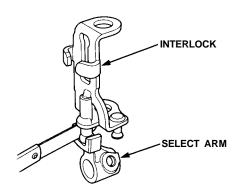
If the clearance exceeds the standard, measure the width of the interlock finger.
