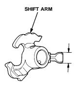
If the width of the shift arm is less than the standard, replace the shift arm with a new one. If the width of the shift arm is within the standard, replace the shift piece with a new one.
