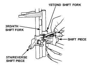
6. If the clearance exceeds the service limit, measure the width of the shift piece.
