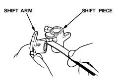
2. If the clearance exceeds the service limit, measure the width of the shift arm.
