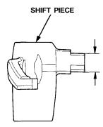
If the width of the shift piece is less than the standard, replace the shift piece with a new one. If the width of the shift piece is within the standard, replace the 5th/reverse shift piece or shift forks with a new one.
