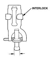
If the width of the interlock is less than the standard, replace the interlock with a new one.
