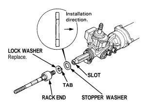
6. Tighten the rack end securely, then bend the lock washer back against the flat on the flange as shown.
