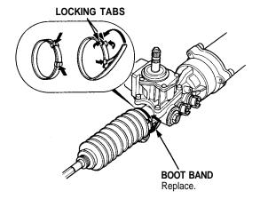
9. If the tie-rod ends were removed, install the tie-rods on the right and left rack ends and screw them in until the threaded section is 11 mm (0.4 in) in length.
