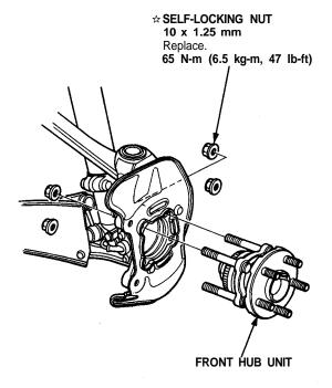
☆: Corrosion resistant bolt/nut
