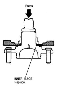
NOTE: Wash the bearing and hub thoroughly in high flash point solvent before reassembly.
