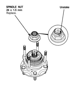
Remove the pulser using a commercially-available bearing puller.
