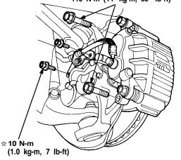
☆: Corrosion resistant bolt/nut
