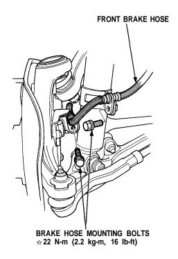
☆: Corrosion resistant bolt/nut
