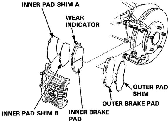
11. Push in the pistons so that the caliper will fit over the brake pads.
