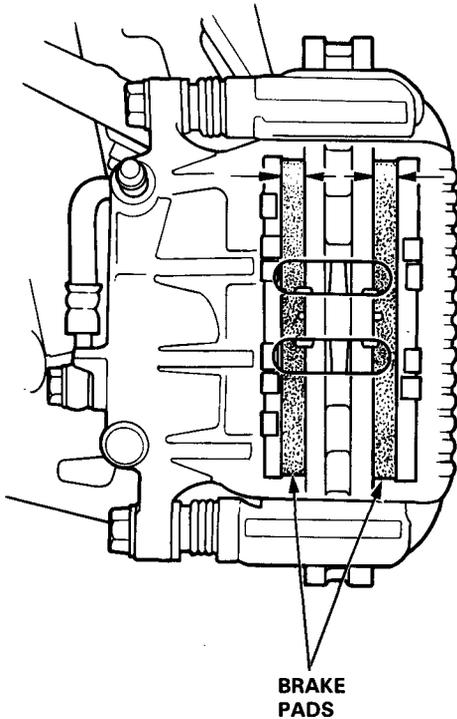
3. Remove the two brake hose mounting bolts. Remove the two caliper mounting bolts, and move the caliper out of the way.
