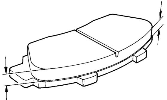
**NOTE:** Measurement does not include pad backing thickness.
