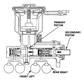
(2) In case of leaking from the secondary system
