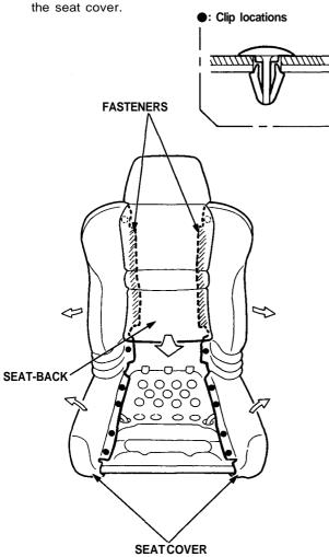
Detach the clips from the seat-back, then pull the seat-back cushion up as shown. Remove the retainers, then remove the headrest by pulling it up. Remove the fastener on the left side.
