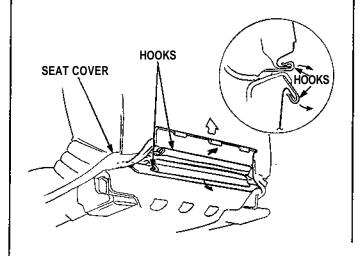
Detach the clips from under the seat, then remove the seat cushion.
