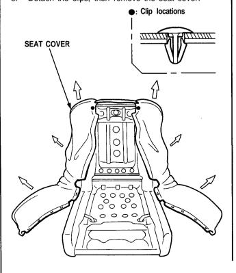
9. Installation is the reverse of the removal procedure.
