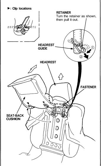
NOTE: When installing the headrest, first install the retainers to the headrest guides.
