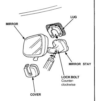
Remove the lock bolt, then remove the toothed lock washer and hold spring from the mirror stay.
