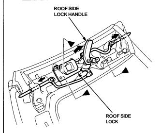
5. Return the roof side lock handle to the unlocked position, then remove it.
