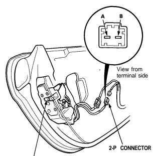
DOOR SWITCH (Built into door lock actuator assembly)
