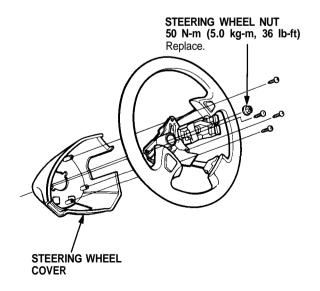
10. Reinstall the steering wheel and the airbag (see section 24).
