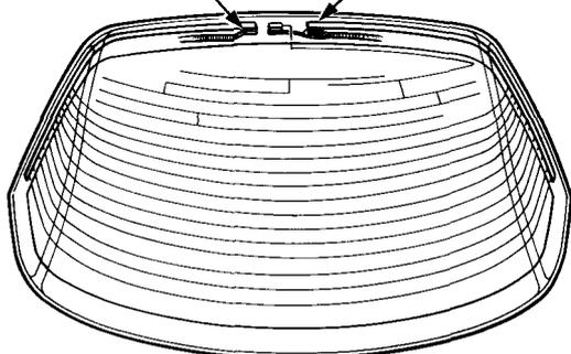
2. Disconnect the positive terminal, check for continuity between the negative terminal and body ground. If there is no continuity, check for an open in the defogger ground wire.
