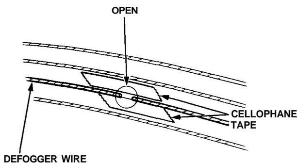
3. Using a small brush, apply a heavy coat of silver conductive paint extending about 1/8" on both sides of the break. Thoroughly mix the paint before use. Let it dry for thirty minutes.
