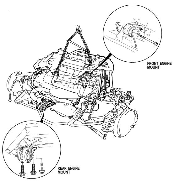
56. Install the engine in the reverse order of removal:
