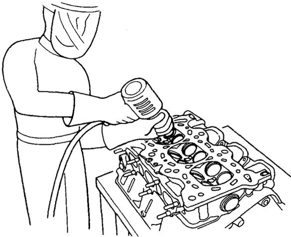
2. Carefully grind a 45° seat, removing only enough material to ensure a smooth and concentric seat.
