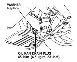
Reinstall the drain plug with a new washer, and refill with the recommended oil.
