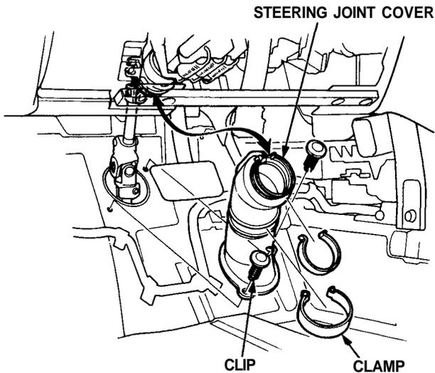
2. Remove the steering joint bolts, and disconnect the steering joint by moving the joint toward the column.
