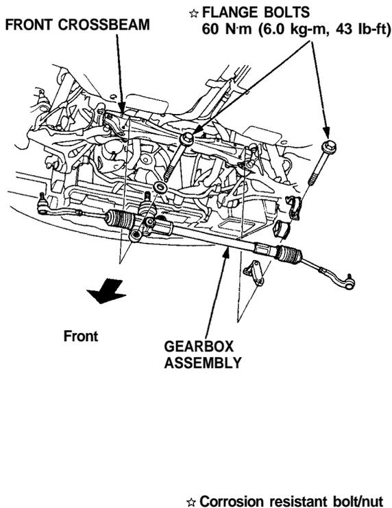
14. Install the gearbox in the reverse order of removal.
