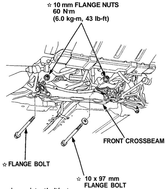
13. Remove the steering gearbox from the front crossbeam by removing the flange bolts.
