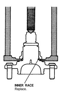
NOTE: Wash the bearing and hub thoroughly in high flash point solvent before reassembly.
