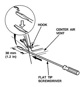
7. Inset the tip of a flat tip screwdriver in under the hook by turning a flat tip screwdriver. Detach the hook by prying it.
