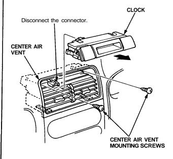
3. Inset a plastic plate between the center air vent and center console panel to prevent damage them.
