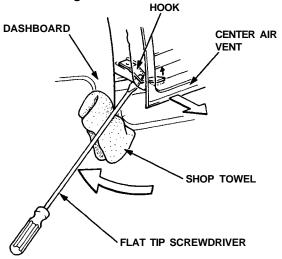
9. Detach the another hook as the same work, then remove the center air vent.
