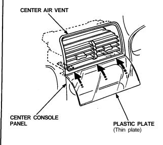
4. To make a gap between the center air vent and dashboard, pull the top of the center air vent while lowering it as shown.
