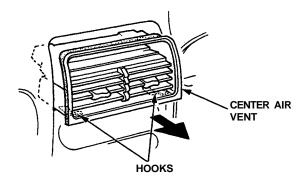
10. Install the center air vent and clock.
