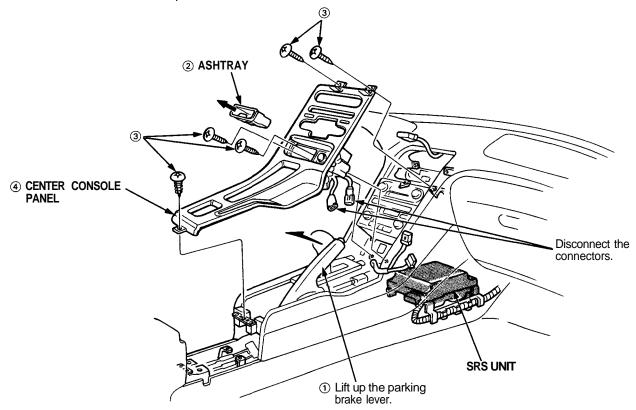
Installation is the reverse of the removal procedure.
