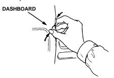
Make sure the connector of the clock is connected properly.
