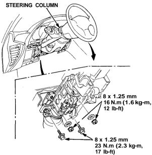
3. Remove the nuts, then remove the airbag bracket (passenger's).
