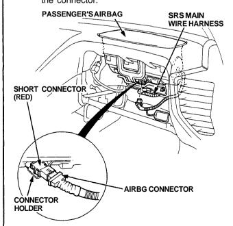
Connect the special tool to the SRS main wire harness connector.
