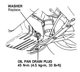
Reinstall the drain plug with a new washer, and refill with the recommended oil.
