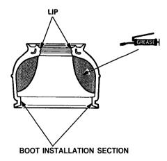
CAUTION: Do not contaminate the boot installation section with grease.
