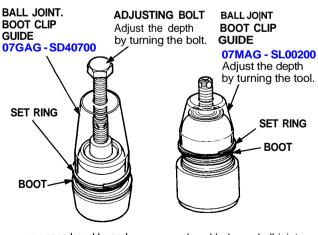
upper knuckle and upper/lower control arm. knuckle lower ball joint only.
