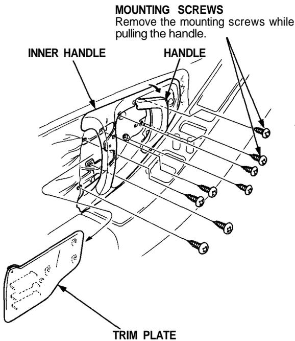
3. Disconnect the connector and handle cable, then remove the inner handle by pulling it forward.
