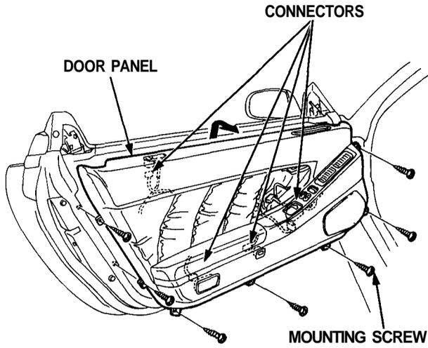
6. Remove the switch panel and air duct from the door panel as required.
