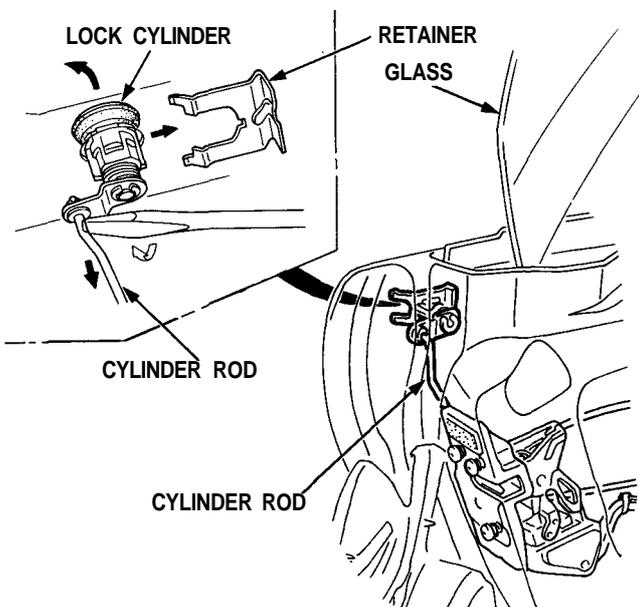
17. Disconnect the lock rod and remove the lock crank. Remove the handle cable and clips. Remove the mounting screws, then remove the latch assembly through the hole in the door.
