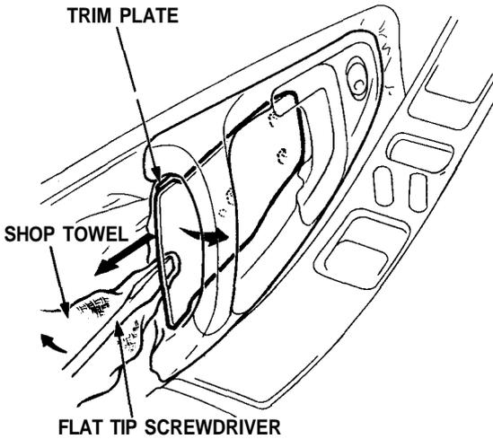
2. Remove the trim plate by pulling it backward, and remove the mounting screws.
