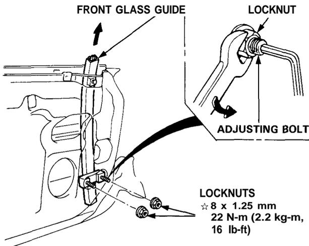
21. Remove the mounting bolts and loosen the motor mounting bolts, then take out the regulator assembly through the window slot.
