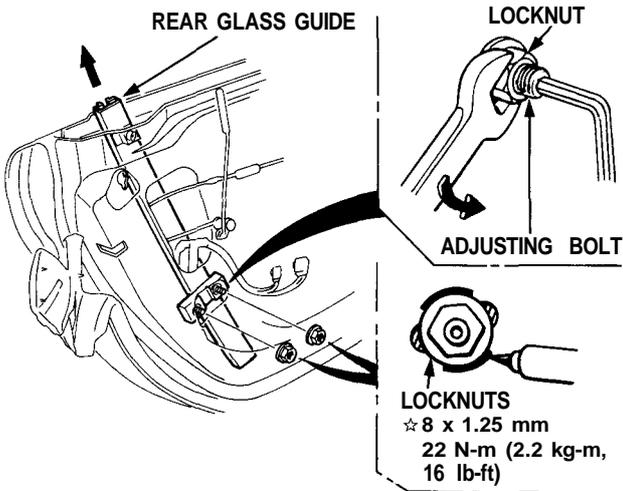
☆: CORROSION RESISTANT BOLT/NUT
