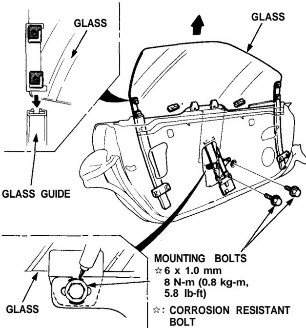
20. Remove the locknuts, then remove the front glass guide.
