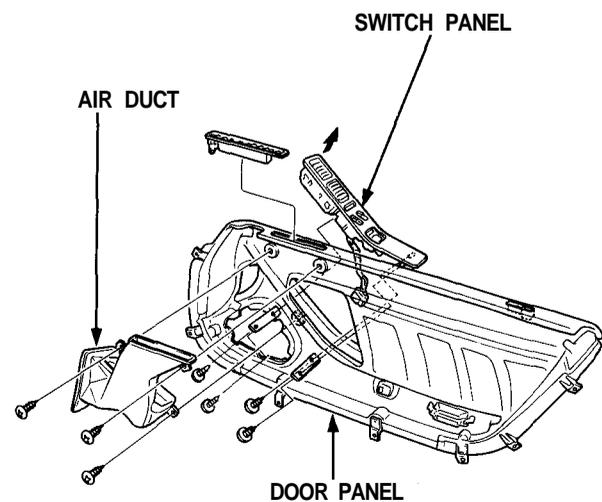
7. Remove the mounting screws and disconnect the connectors, then remove the power window control unit and speaker unit.
