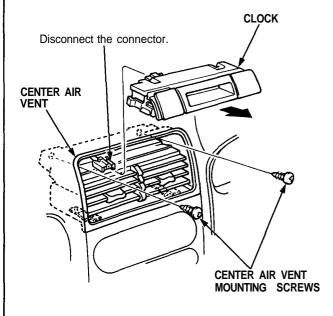
3. Insert a plastic between the center air vent and center console panel to prevent damaging them.
