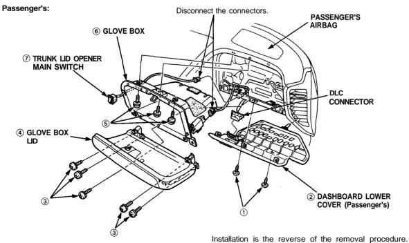
NOTE: Make sure the connectors are connected properly.
