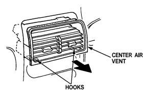
10. Install the center air vent and clock.
