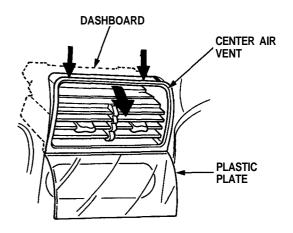
5. Insert a flat tip screwdriver between the center air vent and dashboard as shown.
