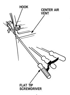
8. Pull the center air vent backward while prying the hook.
