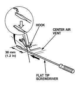
7. Insert the tip the screwdriver in under the hook by pivoting it. Detach the hook by prying it.
