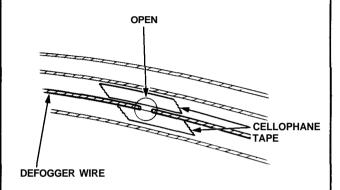
Using a small brush, apply a heavy coat of silver conductive paint extending about 1/8" on both sides of the break. Thoroughly mix the paint before use. Let it dry for thirty minutes.
