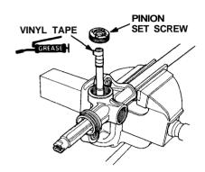
17. Tighten the pinion set screw to a torque wrench reading (indicated) of 9.4—10.4 N·m (94-104kg-cm, 84—93 lb-in).
