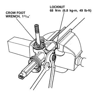
Screw each rack end into the rack while holding the lock washer so its tabs are in the slots in the rack end.
