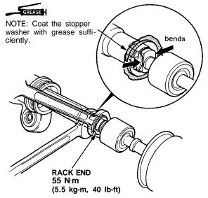
28. Install the boots on the rack end with the tube clamps.
