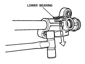
Tap with a plastic hammer to remove the bearing.
