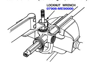
18. Turn the pinion shaft right and left several times to set it, then loosen the pinion set screw.
