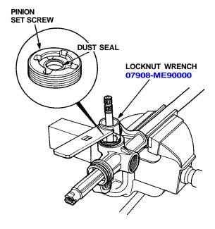
9. Move the rack toward the gearbox side (i.e. in the direction of the arrow) as far as it goes, then pull the steering pinion out when the pinion gear clears the cutout in the rack.
