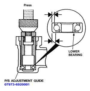
11. Insert the steering rack into the cylinder housing, being careful not to damage the steering rack sliding surface.
