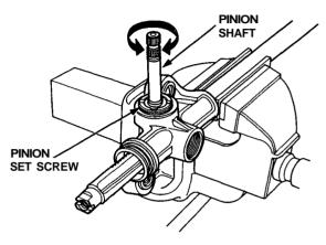
19. Install the special tool onto the pinion shaft. Attach a spring scale to the tool and pull the scale. Adjust the pinion set screw until the gauge reads 1.5—2.5 N (0.15-0.25 kg, 0.33-0.55 lb).
