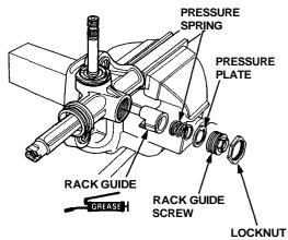
24. Tighten, loosen and retighten the rack guide screw two times to 5 N·m (0.5 kg-m, 3.6 lb-ft), then back it off 15°.
