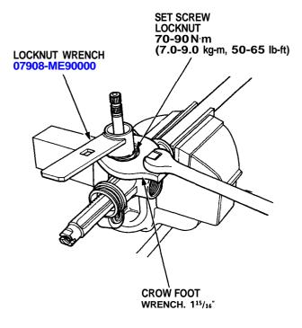
21. Turn the pinion shaft slowly, then insert the rack and engage the rack and pinion gears.
