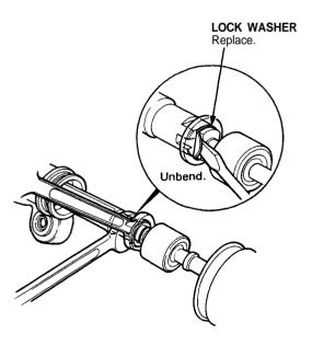
Before disassembly, install the special tool on the pinion shaft and check the preload.
