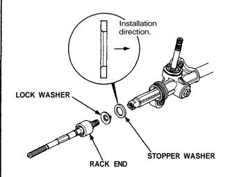
27. Tighten the rack end securely, then bend the lock washer back against the flat on the flange as shown.
