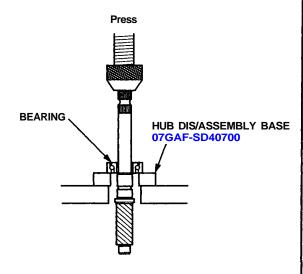
Press the steering pinion into the new pinion bearing.
