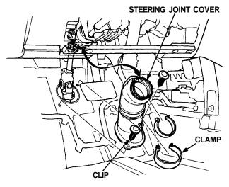
Remove the steering joint bolts, and disconnect the steering joint by moving the joint toward the column.
