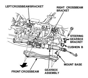
20. When installing the crossbeam to the crossbeam bracket, be sure to align the holes in the crossbeam with the knock pins on the crossbeam bracket.
