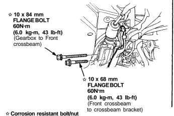
19. Lower the gearbox and front crossbeam with care so as not to interfere with the radiator pipe.
