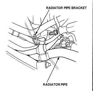
17. Remove the radiator pipe bracket at the floor, and space the radiator pipe away from and gearbox.
