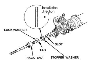
6. Tighten the rack end securely, then band the lock washer back against the flat on the flange as shown.
