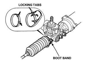
9. If the tie-rod ends were removed, install the tie-rods on the right and left rack ends and screw them in until the threaded section is 11 mm (0.4 in) in length.
