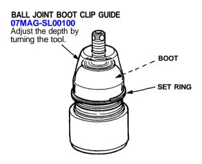
CAUTION: After installing the boot, check the ball pin tapered section for grease. Wipe it if necessary.
