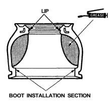
3. Wipe the grease off the sliding surface of the ball pin, then pack the lower area with fresh grease.
