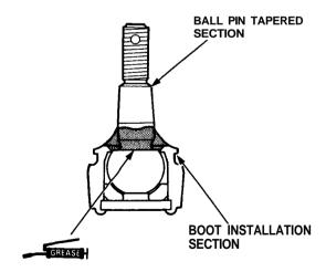
4. Install the boot in the groove of the boot installation section securely, then bleed air.
