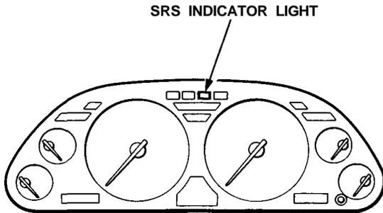
As a system check the SRS light also comes on when the ignition is first turned to the II position. If the light goes off after approximately 6 seconds, the system is OK.
