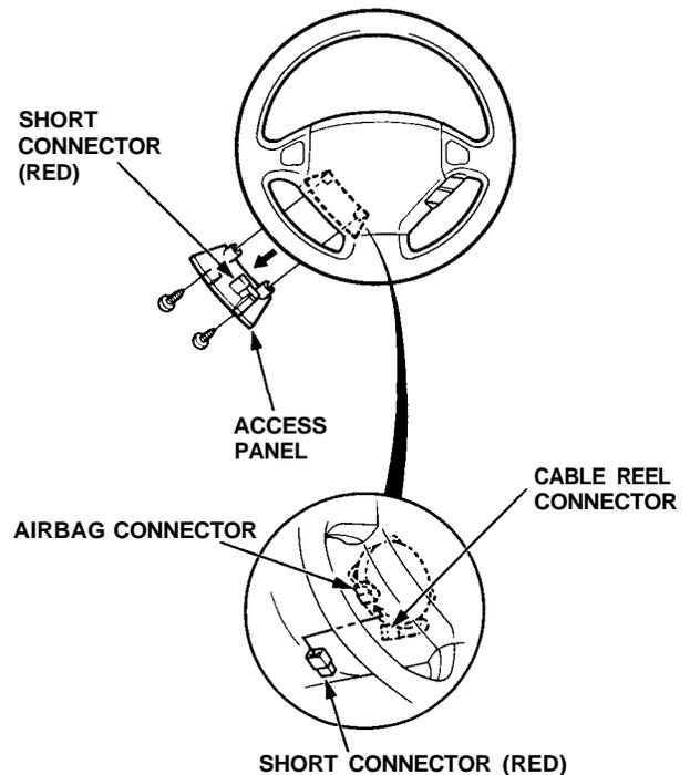
3. Disconnect the connector between the airbag and cable reel, then install the short connector (RED) on the airbag.
